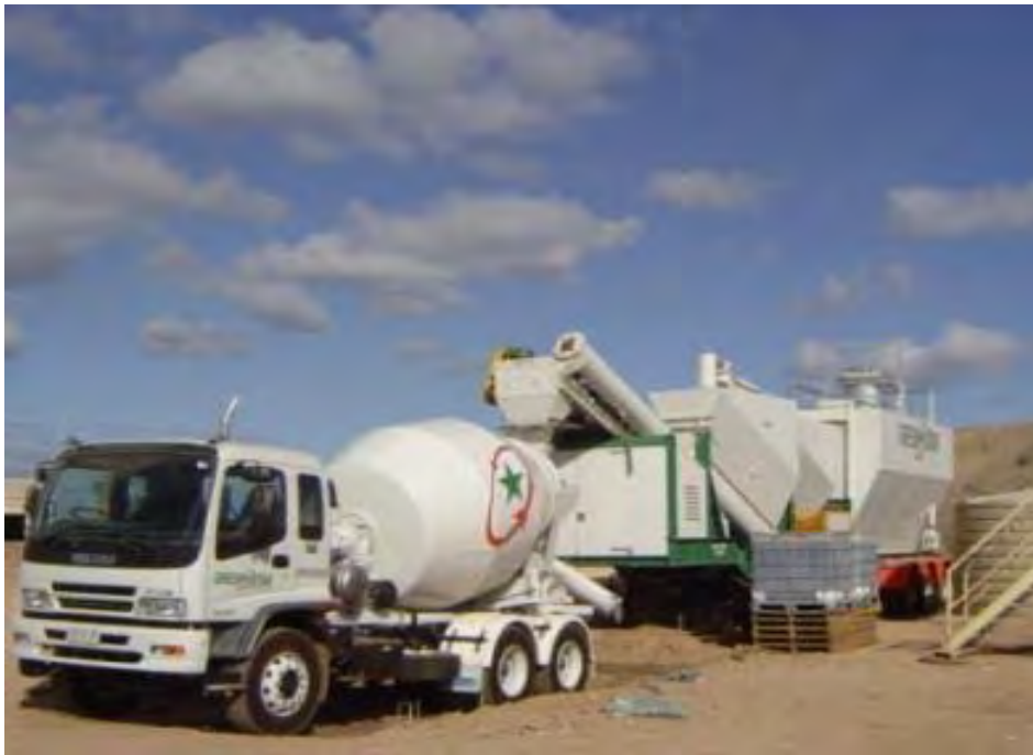
Figure 6 Example – mobile concrete batching plant
