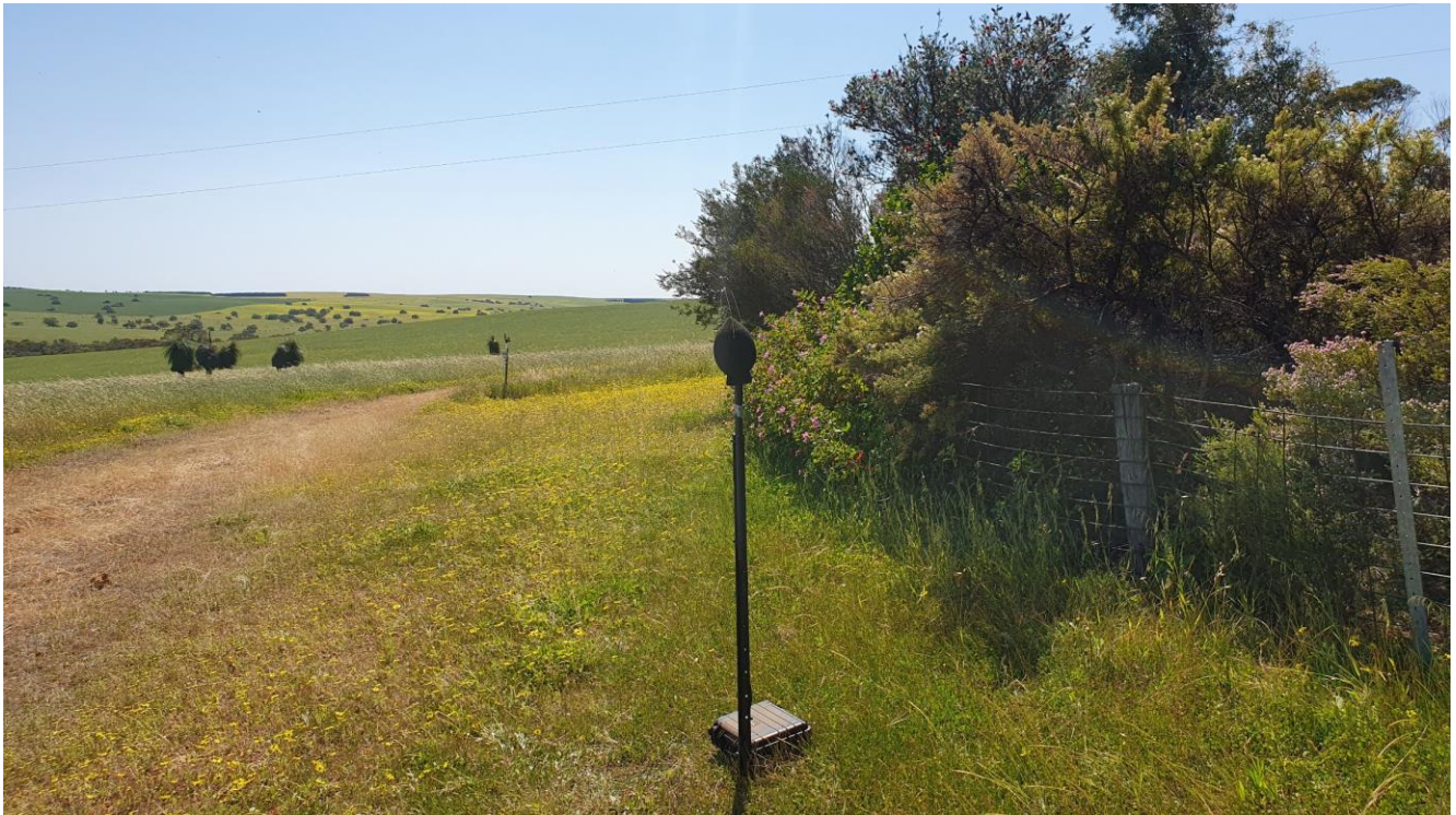
Figure 1: Typical Noise Monitoring Equipment Setup
