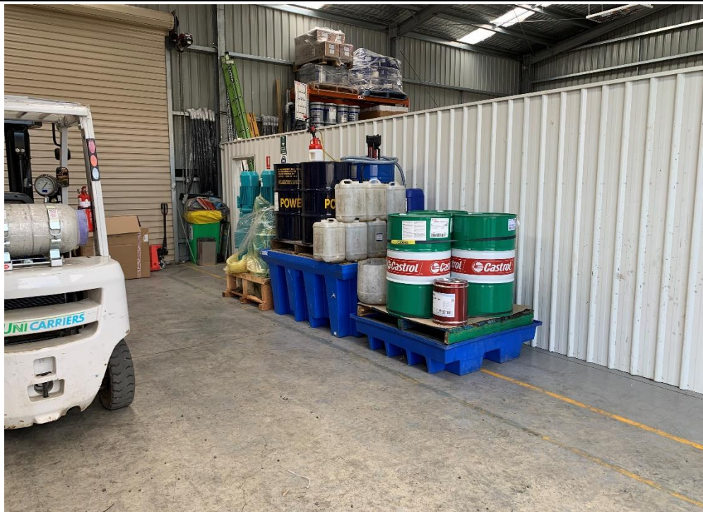
Photo 5: Compound maintenance and storage shed, oils stored on banded pallets in covered and hardstand area.
